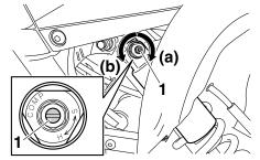
Compression damping force adjusting screw (for slow compression damping) Compression damping setting (for slow compression damping):
