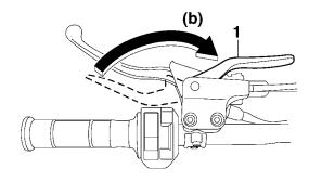
1. Parking brake lever (unlocked position)
