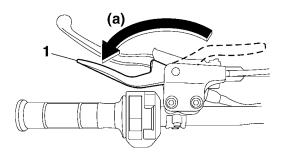
1. Parking brake lever (locked position)
