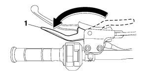
1. Parking brake lever (locked position)
