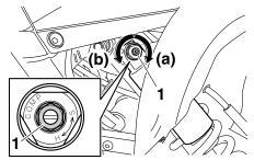
Compression damping force adjusting bolt (for fast compression damping)
