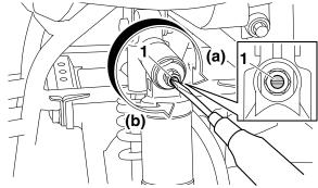
Compression damping force adjusting screw (for slow compression damping) Compression damping setting (for slow compression damping):
