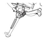
The operation of the sidestand should be checked before each ride, and the sidestand pivot and metal-to-metal contact surfaces should be lubricated if necessary.
